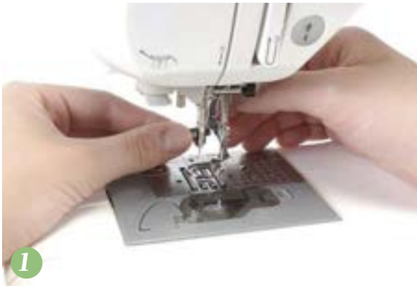
1 Fit your darning foot according to your machine's manual
