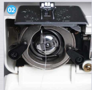
A front-loading bobbin sits inside a metal case
